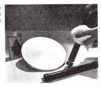
**4** Fit the ink disc to the machine. Check that the ratchet striker engages with the teeth in the underside of the disc.
