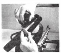
6 With the rollers in their lowest position, grip the chase as shown and lift it upwards and away from the bed. To assist this operation position your fingers in the two depressions at the top of the bed.
