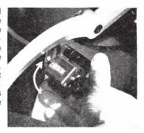
**67** Hold the counter firmly in this position and tighten the grub screw. Do not tighten too much at this stage.
