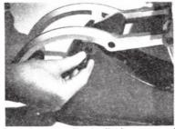
its initial position. When sufficient length of spindle is exposed to view it can easily be withdrawn by hand.
