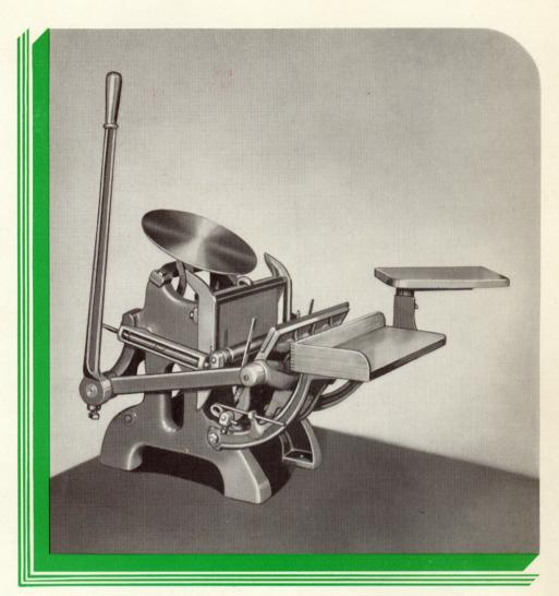
CARDS, tickets, programs, menus and other jobs to be run in small quantities can be printed economically on this thoroughly efficient little press. It is a hand operated press, designed to be mounted on a bench or cabinet. Little or no experience is required in its operation. It is quickly made ready, easily handled and the printing results secured are exceptionally fine for so small a press. The Chandler & Price Company, Cleveland, Ohio.
